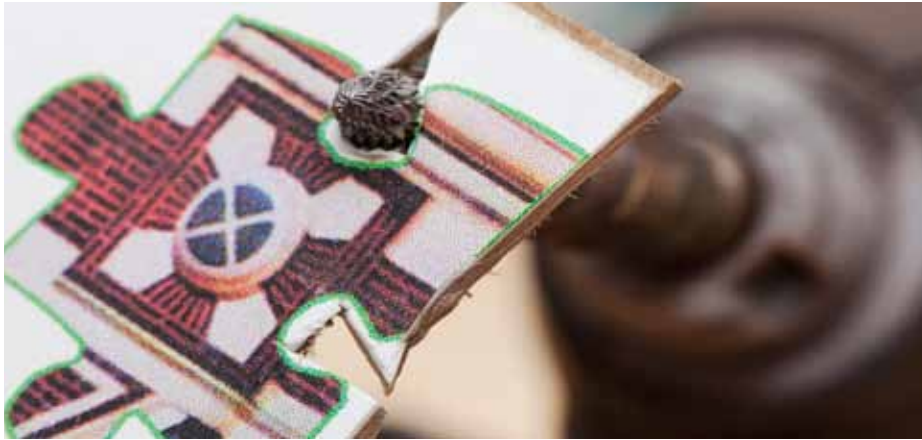
The Dremel grinder with an abrasive burr grinding that triangular hole into a round notch.
